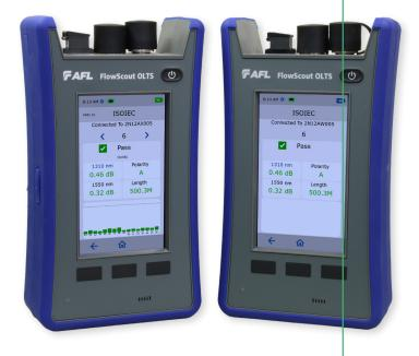
AFL's Flow Scout MPO OLTS is the industry's first true 16-fiber Tier I OLTS tester that supports testing of all multi-fiber AND duplex connectors, enabling much faster test time.
